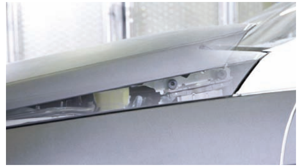
Mercedes-Benz's newly developed Active Bonnet, which enlarges the deformation area, reducing the risk of injury to pedestrians
